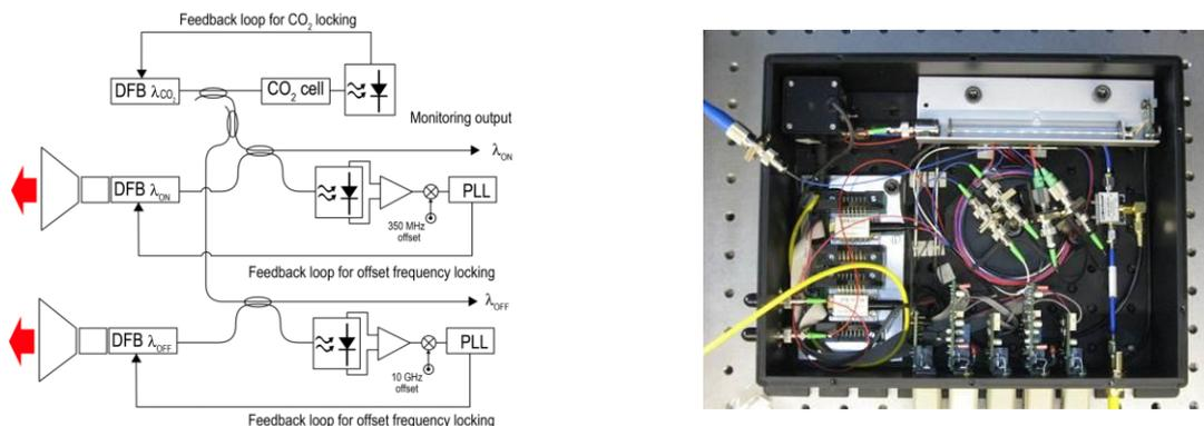
The first design of the Frequency Stabilization Unit (FSU) employs an offset frequency locking scheme referenced to a CO<sub>2</sub> gas cell for frequency stabilization of the two MOPAs inside the BRITESPACE laser transmitter. A first prototype, based on two commercially available lasers is being characterized at ATN.
