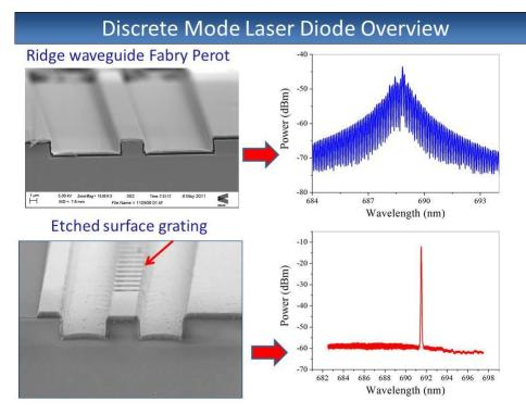
Fig. 1 Electron micrograph of Fabry Perot laser cavity (top left) and Discrete Mode Laser, fabricated by etching a surface grating into the laser ridge (bottom left) along with spectral characteristics of typical visible laser with and without etched filters (top and bottom right respectively)
